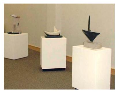
Three pedestals used in an exhibit showing the effect the kick has on the viewer's perceptions. The pedestal at the back has a very low kick while the two in the front have about a four-inch high kick.
